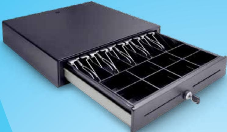
The CHAMP CD 58410 Cash Drawer is designed for more reliable and Secured operations. It is constructed rugged with Thick Gauge cold rolled Steel. Wear resistant Plastic rollers riding on steel guides, provides smooth and Wobble free slide. Its three position lock with a Drawer open sensor offers maximum security for the cash. Adjustable Note Compartment offers flexibility to adjust the width, to accept any currency.
